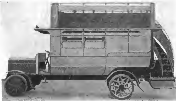
Cedes gearless electric bus with latest type of London body. There are only a few score electric buses in existence in the various European countries and fleets made up of vehicles of this type are unknown there
